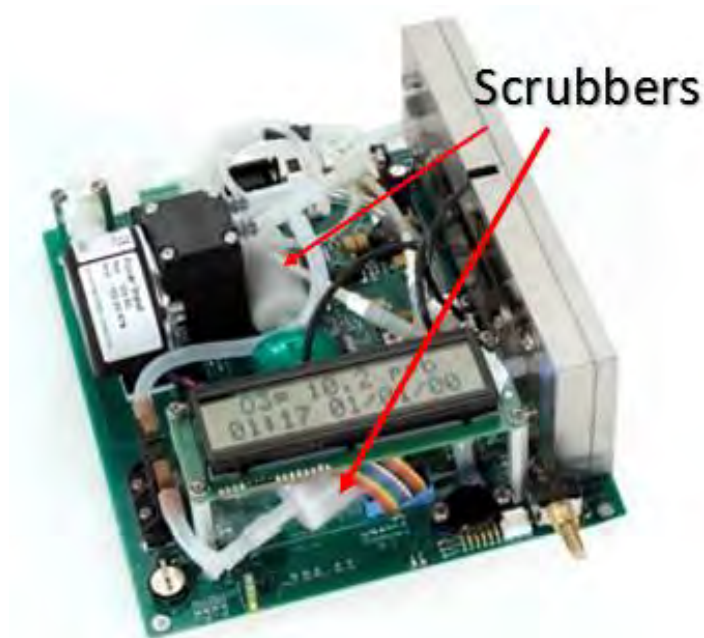
Figure 57. Ozone Scrubber Locations.
